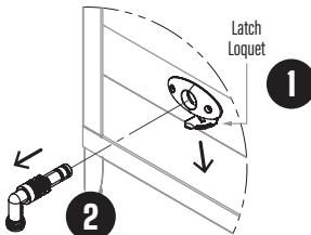
**STEP 2:** Pull to remove the water system block.
