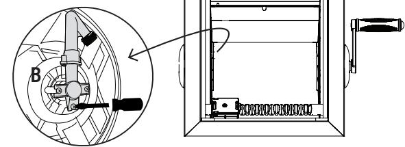
**STEP 6:** Reposition the two drum pieces, aligning the grooves with those on either side. Replace the four screws.
