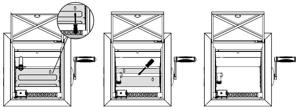
**STEP 5:** Unscrew the three existing water system screws and replace with the new water unit (B).
