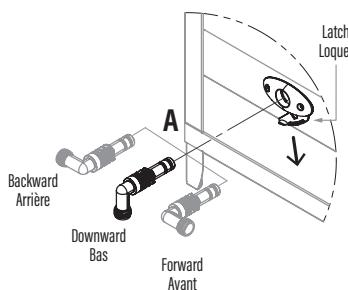
**STEP 3:** Install the new water system bloc (A). The water system block can be directed forward, backward or downward. To install, lower the latch and insert the water system block in the desired direction. Secure by pushing the latch back into its original position.
